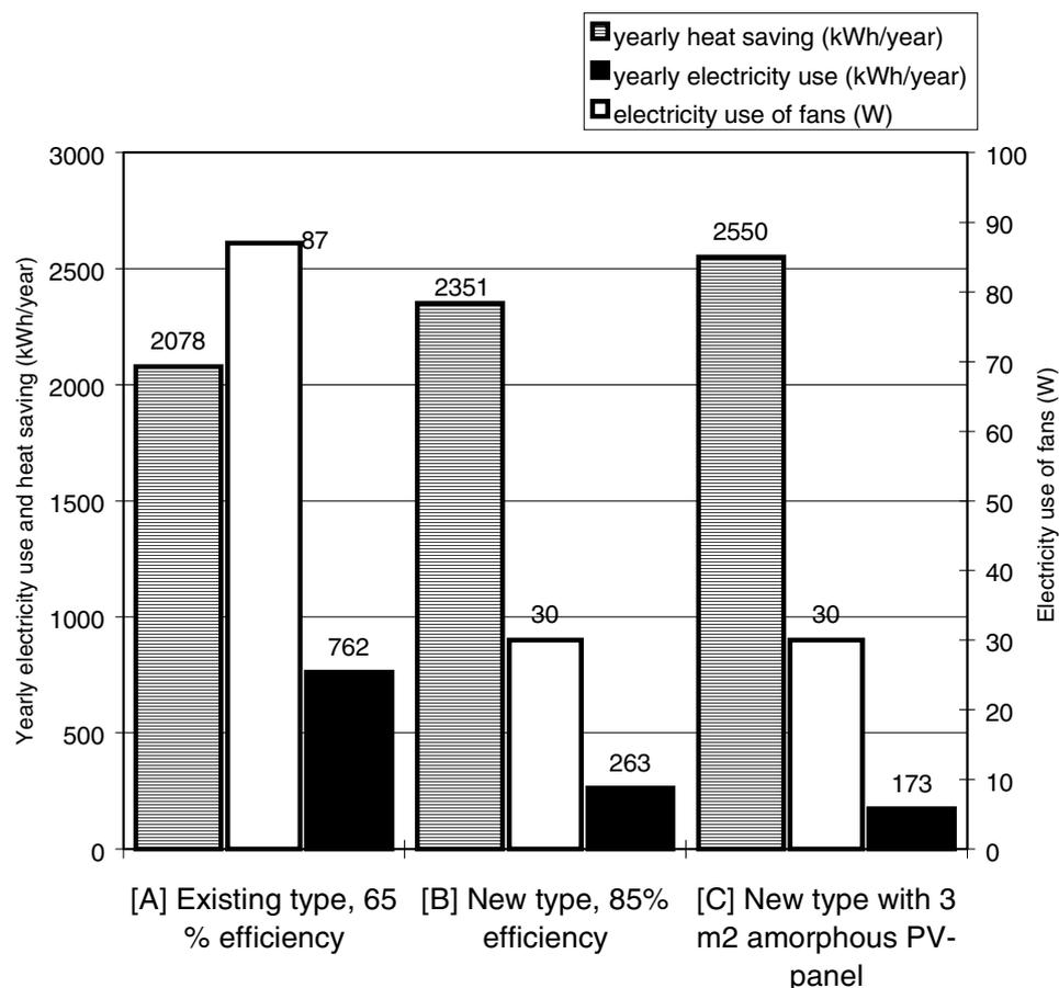
[A] Existing type heat recovery ventilation system (HRV), (cross flow) 65% efficiency, 87 W electricity use according to new Danish Building Regulation (BR95).
